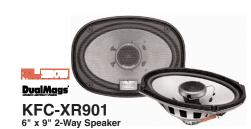
Features •Power Handling 260W •PBO Advanced Fiber Cone Woofer +HyperNyl Dome Tweeter +2-Way Design +Gold Plated Input Terminals Frequency Response: 25Hz - 70kHz Magnet Weight: 2.1 oz x 2 Sensitivity: 93dB/W/m Size (in.): 9-13/16 (W) x 7 (H) x 4-9/16 (D) Mounting Depth: 3-1/16 in Weight: 1.8 lb
